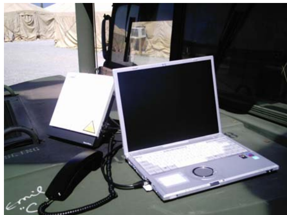
The small satellite modem provides voice and data virtually world-wide.
